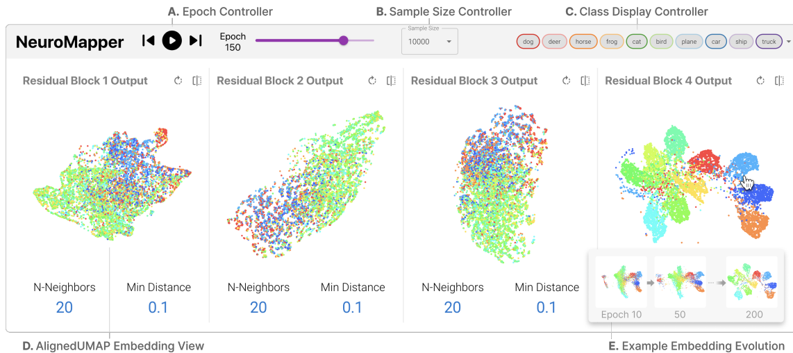
Figure 1: NEUROMAPPER visualizes how a deep neural network (DNN) model, Resnet-50 trained on CIFAR10 dataset in this example, evolves during training by displaying the embeddings for training samples at the model’s blocks throughout the training regiment. A. Epoch Controller for updating the embedding display by adjusting the training epoch through a slider or auto-incrementation using the controller. B. Sample Size Controller changes the number of samples. C. Class Display Controller toggles classes’ sample visibility. D. AlignedUMAP Embedding View visualizes input embeddings represented by each block in the DNN model, with user-adjustable hyperparameters at the bottom. E. Example Embedding Evolution of the fourth residual block of the model at epochs 10, 50, and 200.
